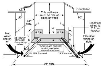
**Note:** Dishwasher must not be installed more than 10' from sink for proper drainage. All plumbing and electrical work must be in accordance with local codes. Dishwasher includes drain hose and leveling legs.
